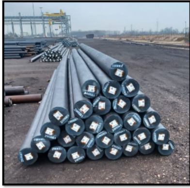
Fig. 1 Illustration of the products' positions with QR code tags
