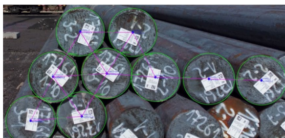
Fig. 6 Outdoor QR detection: (left) circle and QR detection; (right) position graph overlay
