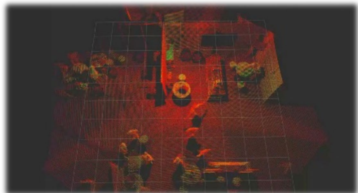
Fig. 4 Illustration of an obstacle that generates occlusions in both LiDAR mirrors
